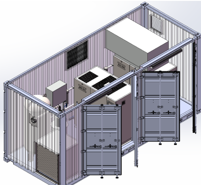
Air compressor station module
